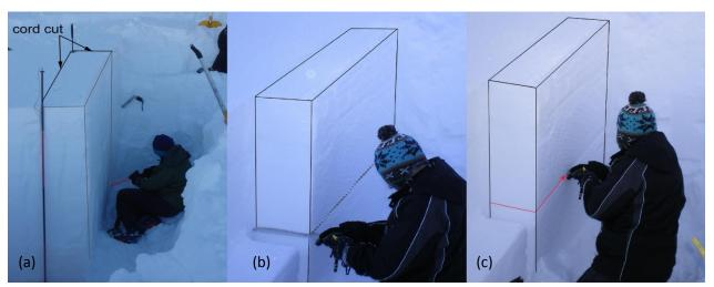
**The PST process:** (a) isolating the column using probes and cord; (b) identifying the weak layer and preparing to cut; (c) saw-cutting the weak layer until the fracture propagates ahead of the saw.
