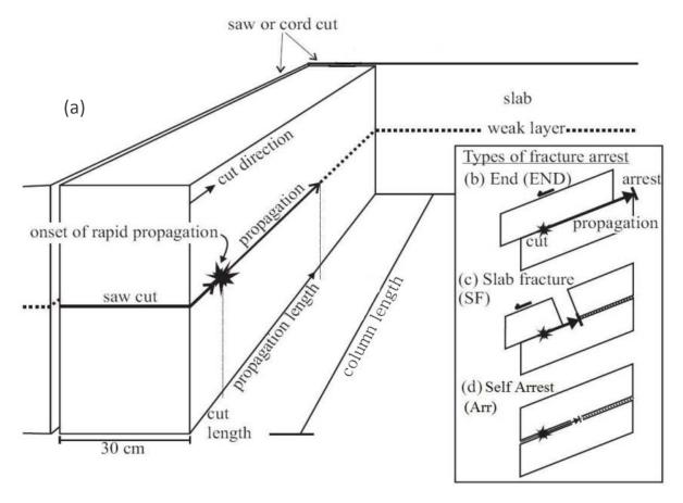
**PST Schematic:** The PST column is shown (a) with the three possible observable results of propagation to end (b), slab fracture (c), and self arrest (d)
